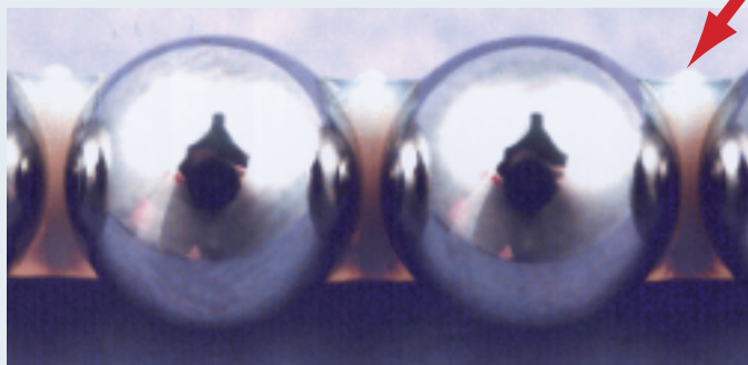
Contact state between balls and ball cage
