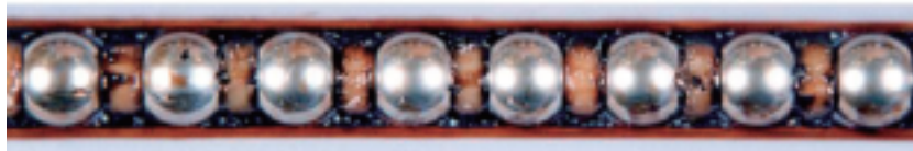
Ball cage after running 8,000 km (Test stop)
