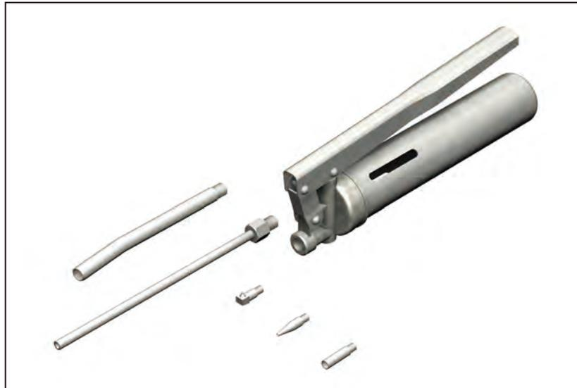
The grease gun unit MG70 is capable of supplying grease for SKR/KR by replacing the dedicated nozzle. The grease gun has a slit window that allows you to visually check the remaining amount of grease. Since grease is contained in a 70 g bellows cartridge, you can replace the nozzle without soiling your hand.
