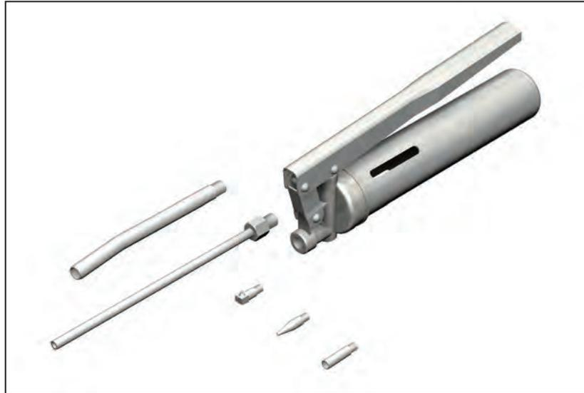
The grease gun unit MG70 is capable of supplying grease to TH20 and TH25 models by replacing the dedicated nozzle. The grease gun has a slit window that allows you to visually check the remaining amount of grease. Since grease is contained in a 70 g bellows cartridge, you can replace the nozzle without soiling your hand.
